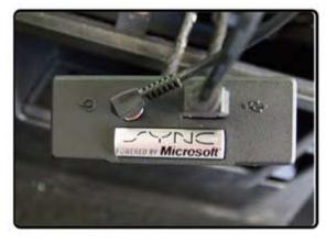
Connect the cables to the corresponding SYNC connections and secure them.
