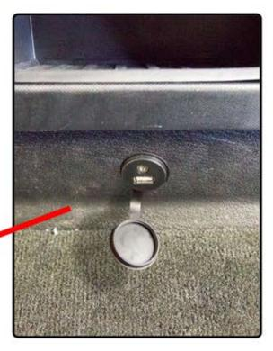
Mount the new extension port and run the cables behind the headunit.
