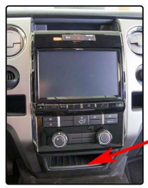
Trim the plastic below the pocket in vehicles without a center console according to the 3rd party extension of your choice. If vehicle has a center console place the after market extension ports inside of it. (see 3rd party parts image below)
