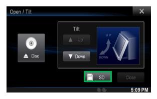
4.3) Insert the updated SD card into the head units SD card slot then select "Close".
