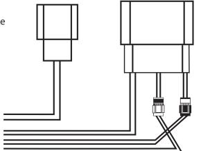
Premium audio system you must remove the speaker pins and relocate them like shown on the picture above.
