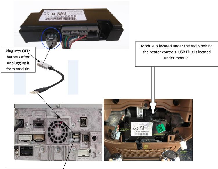
Plug the Alpine USB Interface ' into the USB input on the back of the X009-WRA using supplied extension cable.
