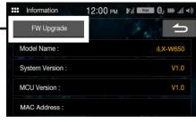
3-4 Push FW Upgrade. This process should take about 2 minutes. The head unit will reboot when the update has finished.
