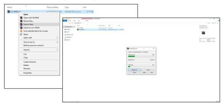
2-2 Once extracted you will see a folder named iLX-W650. Copy the unzipped folder to your flash drive by copy and pasting or dragging and dropping the file. The pictures below show the folder iLX-W650 on the flash drive and the folders in it. Note: You can NOT change the file names or folder names. The head unit will not recognize the files if you do. DO NOT just copy the files to the drive. You need to copy the folder.
