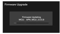
3-5 The firmware update screen will automatically change and do the next part of the update. The head unit will reboot when the update has finished. Remove the thumb drive from the USB port. Go back to the SYSTEM menu and press RESET to do a hard reset which will restore everything to the factory default settings. If there's settings that you have changed then please make note of them before doing the reset. Yes, the hard reset is a necessary step.
