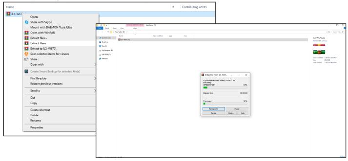
2-2 Once extracted you will have 3 files named ISPBOOOT.BIN, ISPBOOOT.md5, and mcuupdate.hex. Copy just those files to your flash drive by copy and pasting or dragging and dropping the files. The pictures below show just the root of the thumb drive with only the files in it. Note: You can NOT change the file names or folder names. The head unit will not recognize the files if you do. DO NOT put the files into another folder and copy that. You must copy only the files.
