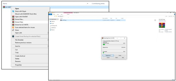
2-2 Once extracted you will have 3 files named ISPBOOOT.BIN, ISPBOOOT.md5, and mcuupdate.hex. Copy just those files to your flash drive by copy and pasting or dragging and dropping the files. The pictures below show just the root of the thumb drive with only the files in it. Note: You can NOT change the file names or folder names. The head unit will not recognize the files if you do. DO NOT put the files into another folder and copy that. You must copy only the files.
