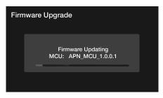
3-5 The firmware update screen will automatically change and do the next part of the update. The head unit will reboot when the update has finished. Remove the thumb drive from the USB port. Go back to the SYSTEM menu and press RESET to do a hard reset which will restore everything to the factory default settings. If there's settings that you have changed then please make note of them before doing the reset. Yes, the hard reset is a necessary step.
